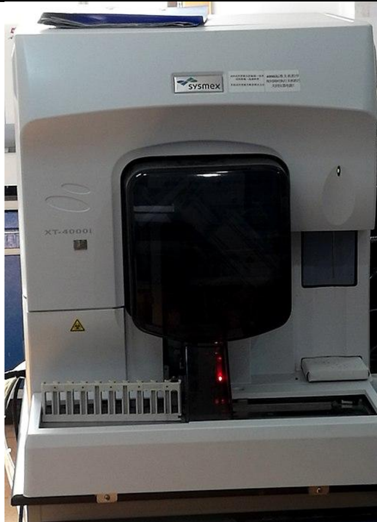
Figure 3 Automated laboratory analyzer handling blood and test tubes. Such systems perform high-throughput assays
