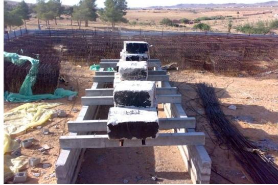
Figure (2-a). Beam's loading technique
