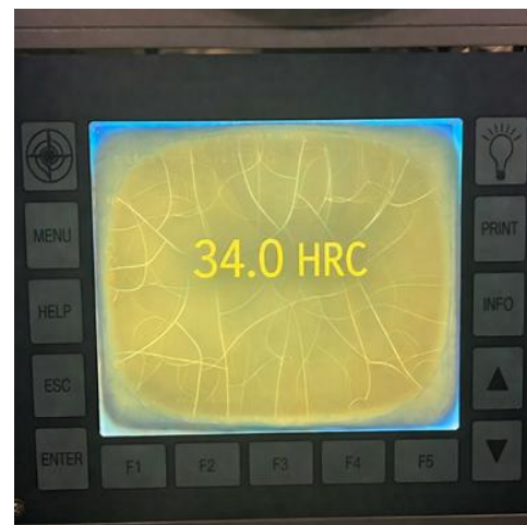
Figure 4. Hardness measurement showing 34 & 36HRC.
