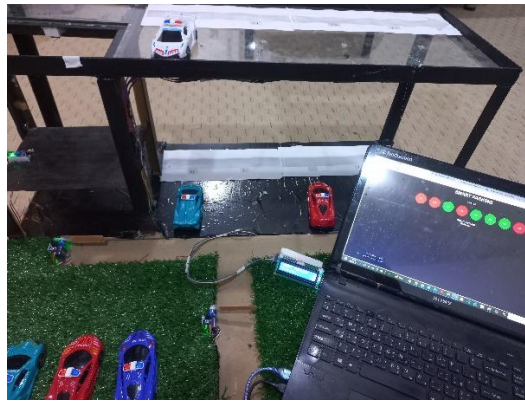
Figure 16. Parking System with Available Parking slots.
