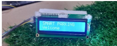
Figure 11. shown used LCD to guide drivers to the appropriate parking place
