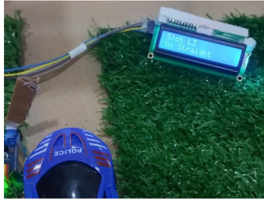
Figure 20. Driver guidance to an available parking slots L3 on lower level
