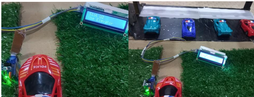
Figure 20. Figure 21: Driver guidance to an available parking slots L3 on upper level
