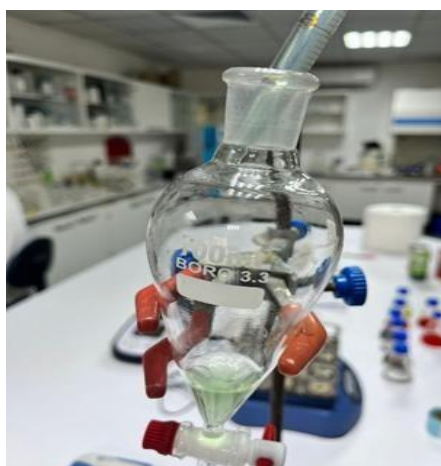
Figure 2. Sample Preparation for the Determination of Sodium Benzoate
